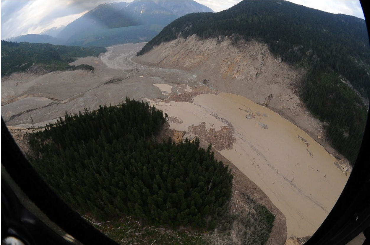
Figure B-7. Landslide dam on Meager Creek from the August 6, 2010 rockslide-debris flow from Capricorn Creek. The dam impounded Meager Creek for some time. Photo by D. Steers.
