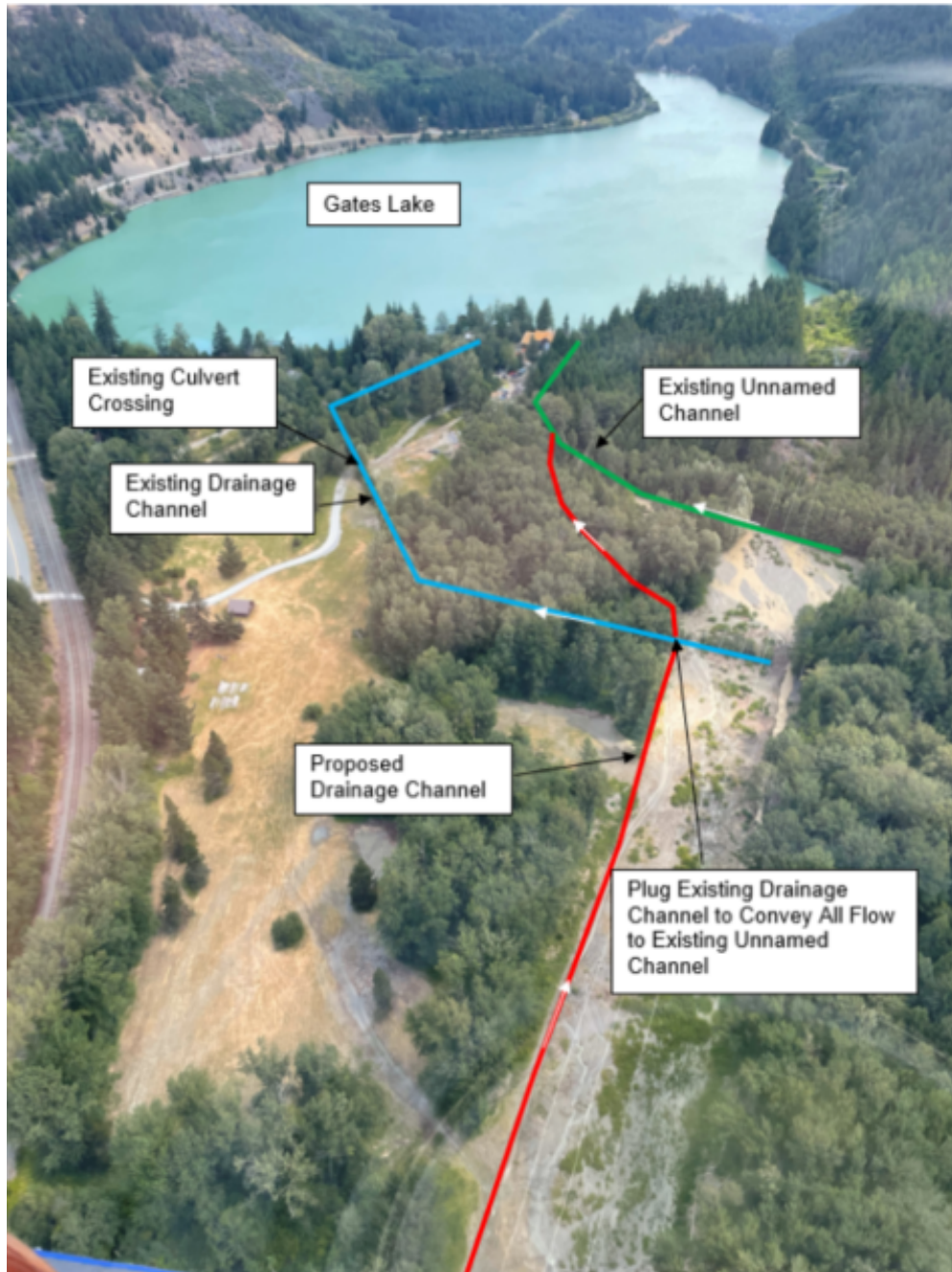
Figure 23 – Emergency Flood Mitigation Works Plan Implemented from Aug 1 to 8 th
