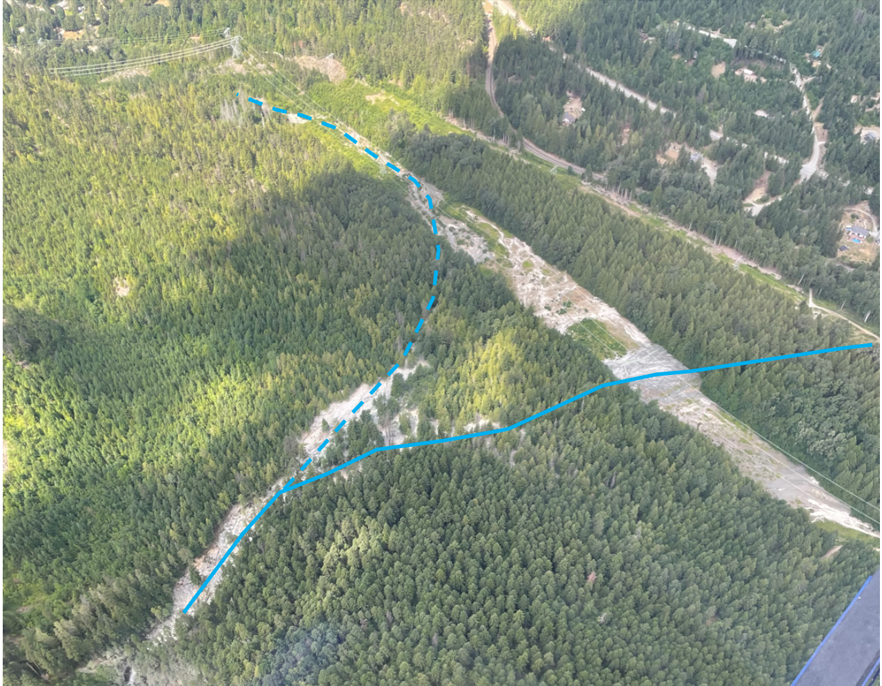
Figure 6 - Place Creek Post-Event (Solid Line) and Pre-Event (Dashed Line) Alignments (Stantec, July 24, 2024)
