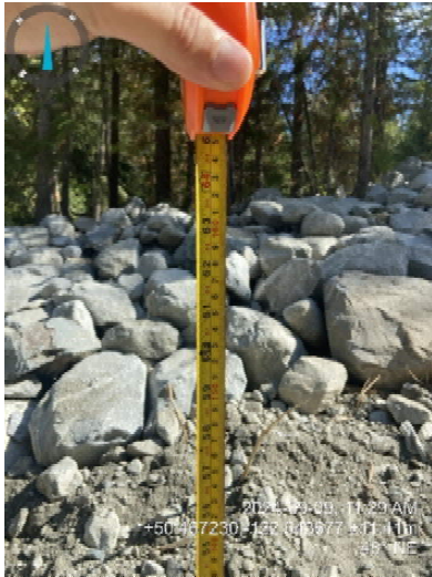
Image 6: channel depth measured to be 1.6 m (2024-09-09 @ 11:29 AM)
